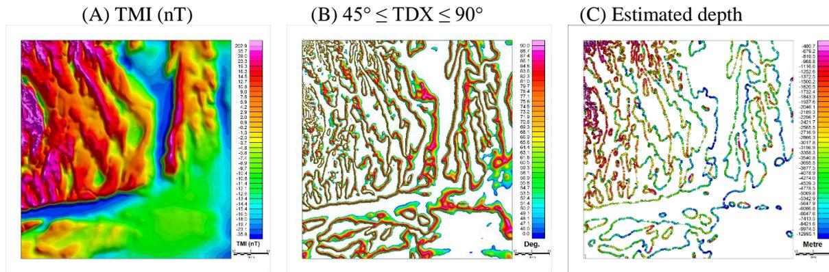
**Figure 3** Bishop Models. (A) TMI response generated from a basement model, with uniform magnetic basement susceptibility, RTP'ed, and field strength of 50,000nT (B) TDX map showing contour of interest ( $45^\circ \leq \text{TDX} \leq 90^\circ$ ) (C) Estimated depth along the edge.
