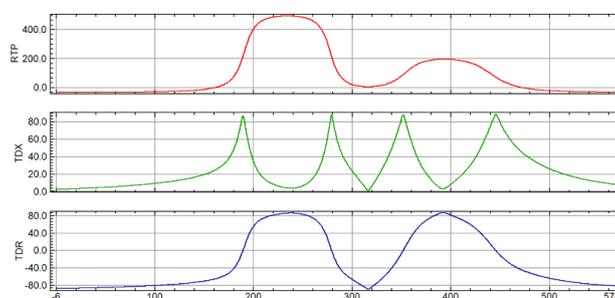
**Figure 2** Comparison of TDX and TDR profile response over the two magnetic prism blocks in Figure 1. The vertical lines represent the contact or edge boundary. **Maxima** from the TDX and **zero crossing** from the TDR.
