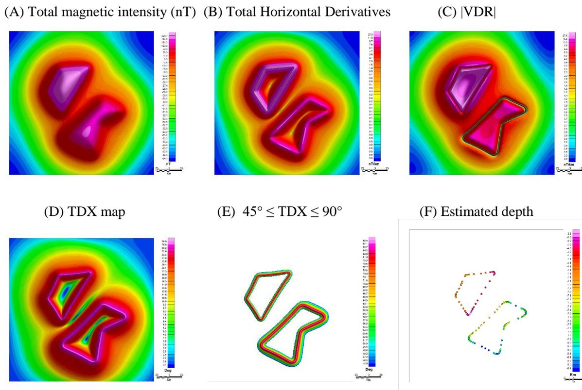
**Figure 1** Two prism Model (A) TMI (B) Total Horizontal Derivative (C) Absolute value of Vertical Derivative (D) TDX map and (E) contour of interest,  $45^\circ \leq TDX \leq 90^\circ$  (F) Estimated depth along the depth of the block.
